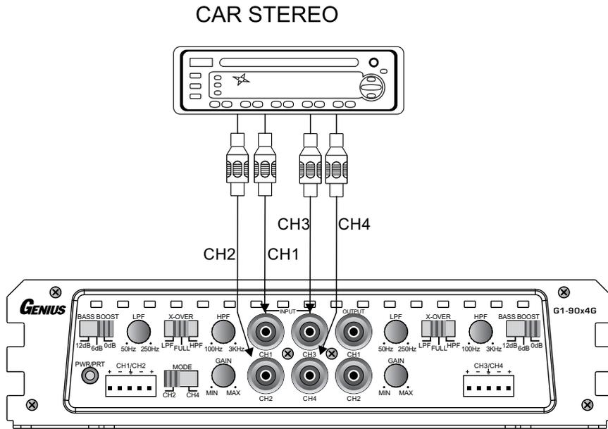
**Low level input:** These are driven by the line output of your in dash radio or intermediate signal processor, Separate Left and Right signals can be applied for Stereo or Mono operation but both inputs must be driven with the same signal for proper Bridged operation. If only mono signal is available, a "Y" adapter is required.
