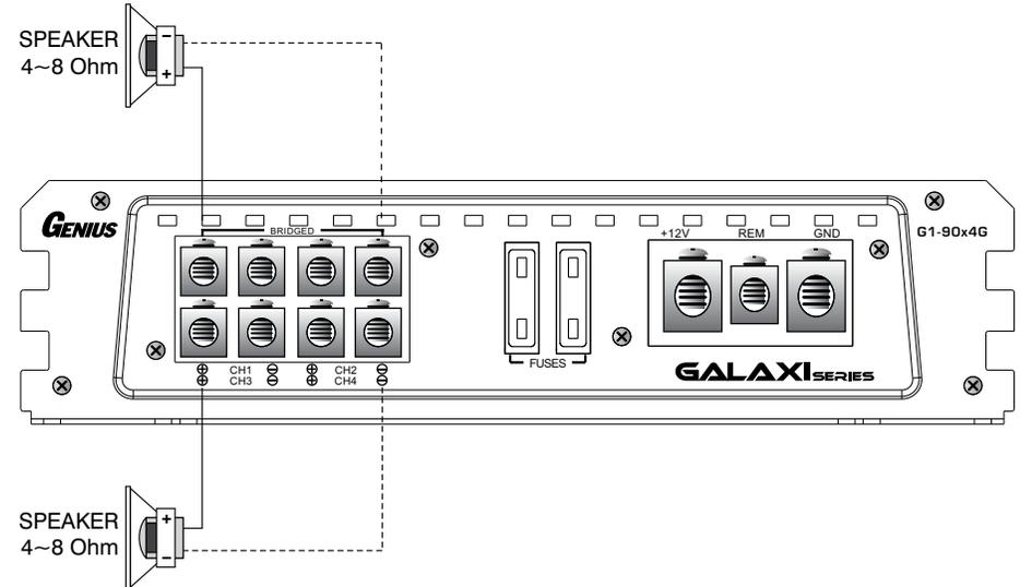
Note that the four speakers have been connected to the four terminal following the (+) and (-) graphic. Your speaker terminals may be marked (+) and (-) or there may be a red dot by one terminal which means the same as (+).
